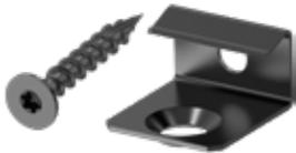
**PENETRATION DEPTH** MINIMUM deck board groove should be 1/8" tall x 1/4" deep. The material remaining below groove (dim A) must be at least 1/4". The bottom of the plastic part of the clip is not designed to contact the joist. See image to the right for a visual representation of the clip's gusset and screw.
