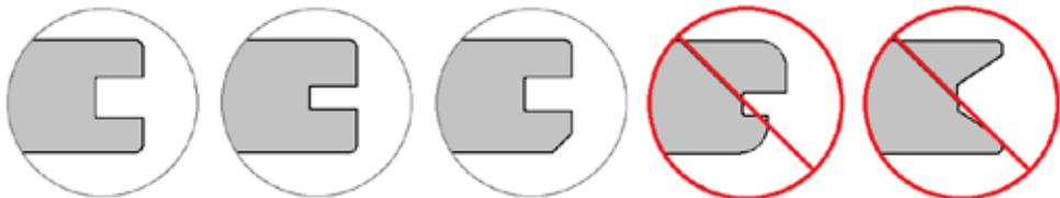
**PENETRATION DEPTH** MINIMUM deck board groove should be 1/8" tall x 1/4" deep. The material remaining below groove (dim A) must be at least 1/4". The bottom of the plastic part of the clip is not designed to contact the joist. See image to the right for a visual representation of the clip's gusset and screw.
